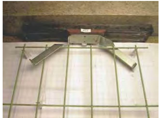
Fig. (11). Picture showing orientation with respect to steel reinforcing mesh for connectors with offset legs (as indicated in Table 1).
