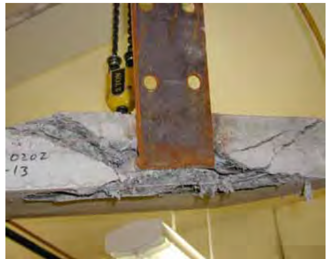
Fig. (12d). Concrete slab damage sustained as a result of testing Connector C in vertical reversed cyclic shear.
