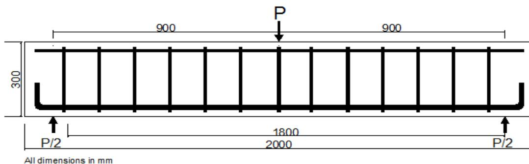
Fig. (1). Specimens details of B1.
