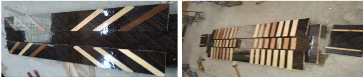
Fig. (4). Preparations of molds for vertical and inclined CFRP for B4 and B5.
