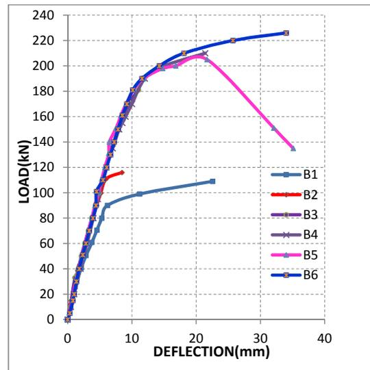
**Fig. (6).** Load-deflection of all specimens.
