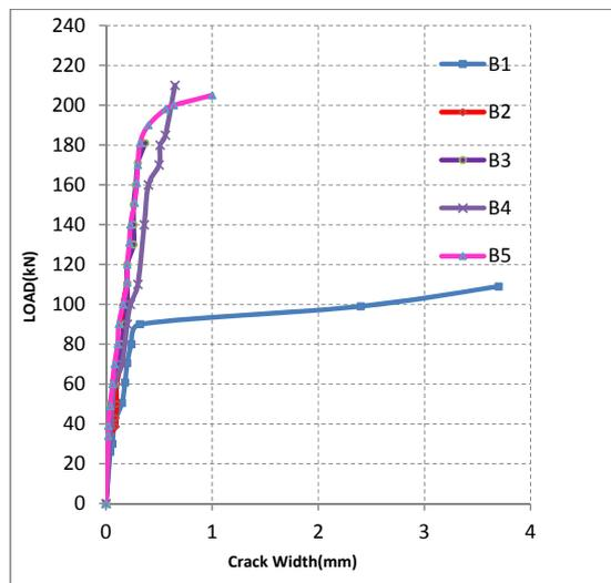
Fig. (7). Load-crack width of all specimens.
