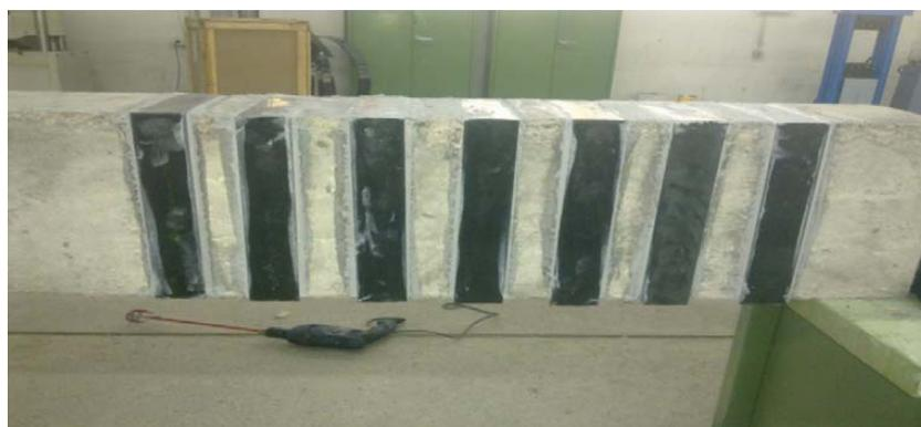
Fig. (5). Placing of vertical CFRP strip (embedded near surface) for B4.
