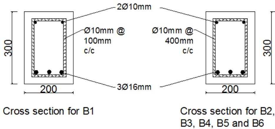
Fig (2). Cross section of specimens.
