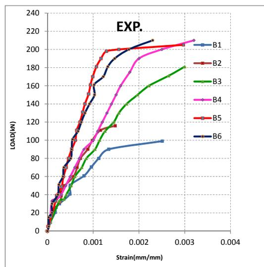
Fig. (8). Load-compression strain of all specimens.
