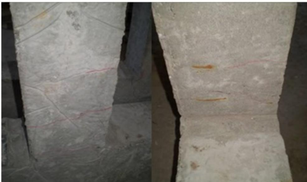
Fig. (10). Crack development of No.3 specimen in the cyclic load.
