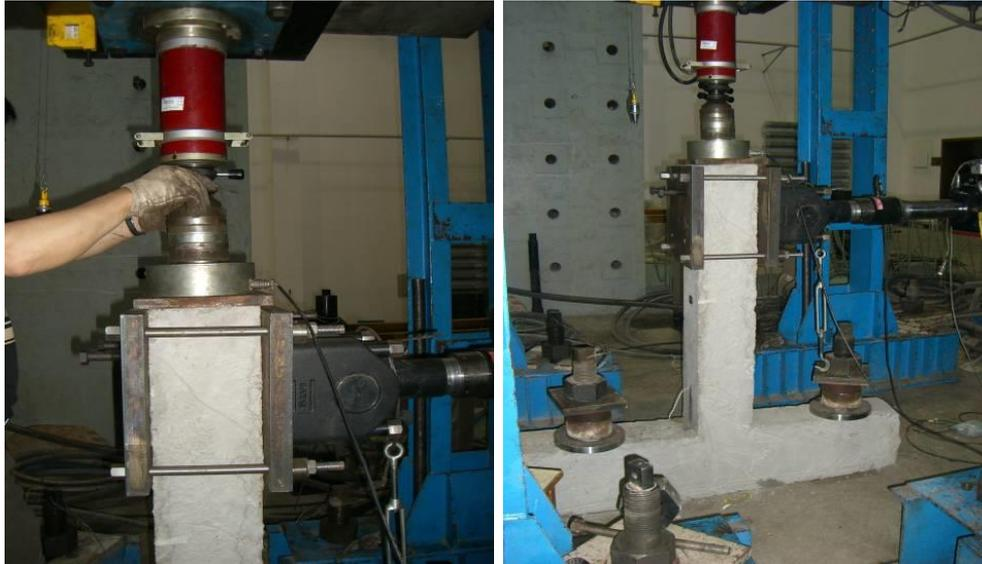
**Fig. (7).** Fixture and specimen installation.
