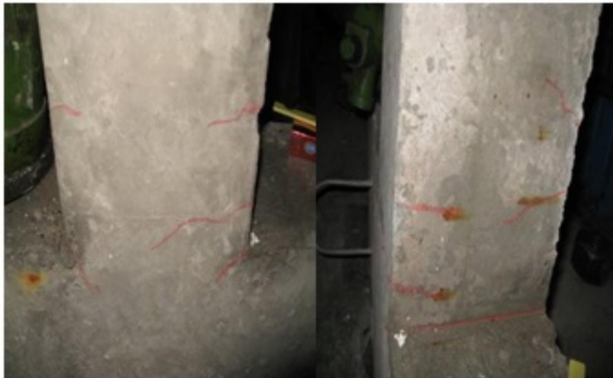
**Fig. (11).** Crack development of No.4 specimen in the cyclic load.
