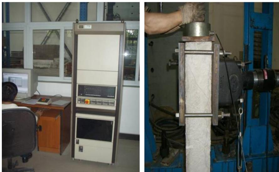
**Fig. (4).** MTS system and data collection system.
