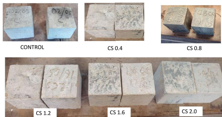
Fig. (17). Concrete surface after ponding in sodium hydroxide solution.
