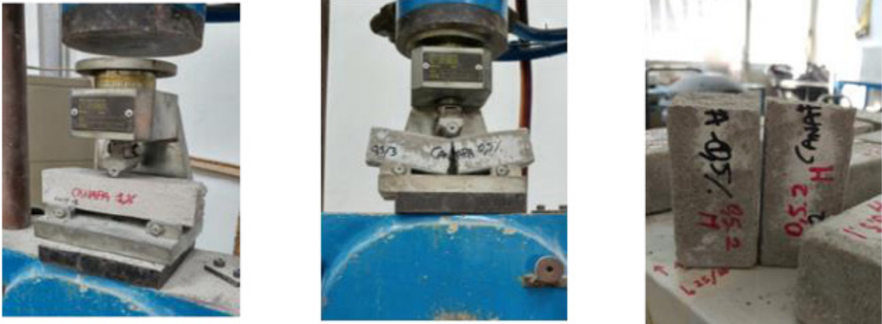
Fig. (8). Bending test phases.
