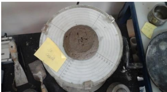
Fig. (3). Shaking table on the additive mixture.
