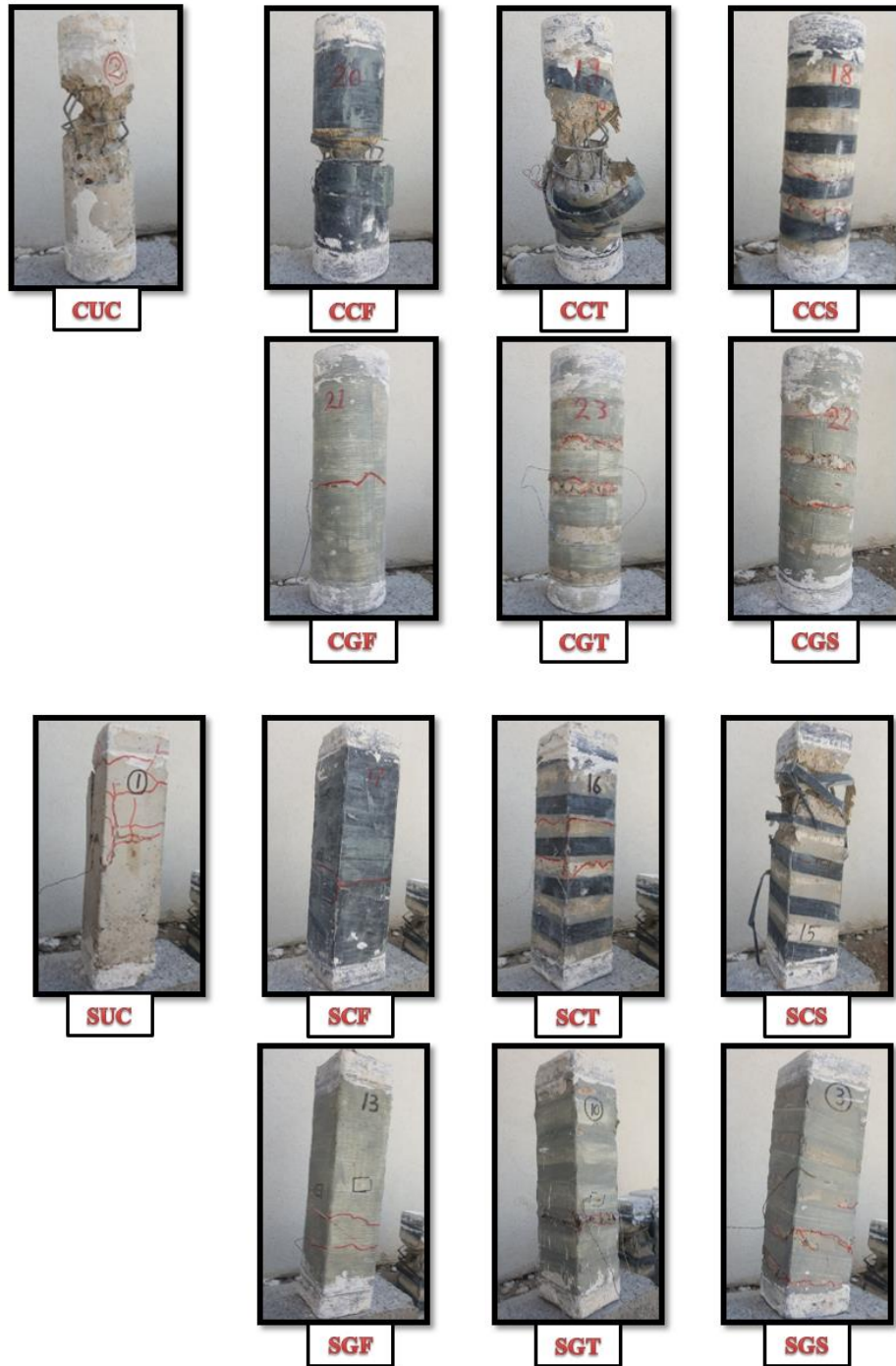
Fig. (3). Crack patterns for Columns G1- G4 at ultimate loads.
