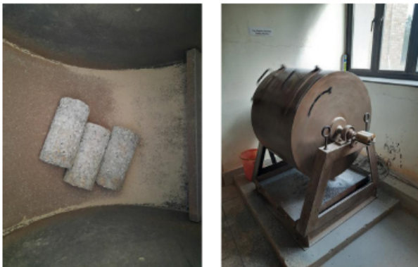
Fig. (9). Cantabro test for abrasion resistance.
