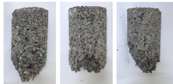
Fig. (19). Failed specimens indicating crushing of bottom layer.
