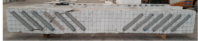
Fig. (21). The strengthened beam using GFRP.
