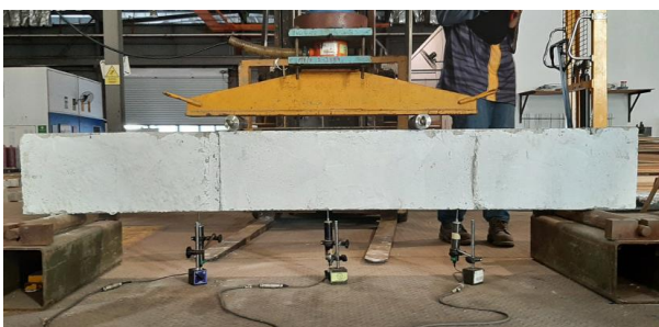
Fig. (13). Four-point bending test on the control beam.
