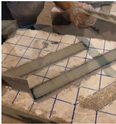
Fig. (8d). The GFRP strips were filled with adhesive and later pasted on the RC beam.
