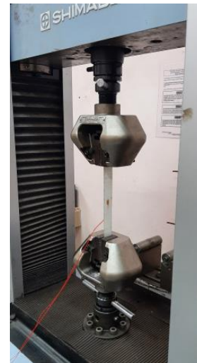
Fig. (10). Tensile test conducted on the GFRP strips.
