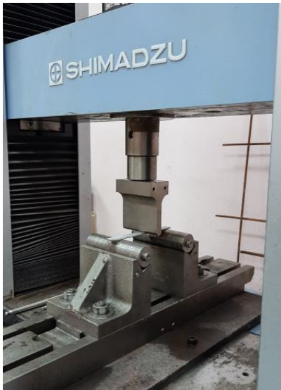
Fig. (12). Flexural test conducted on the GFRP strips.
