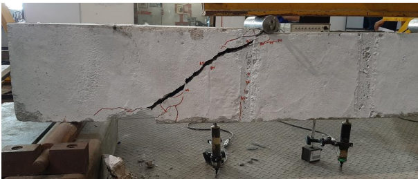
Fig. (19). Crack pattern of the control beam.
