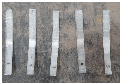
Fig. (17). Failure mode of the GFRP strips in flexural.
