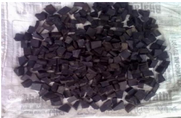
Fig. (2). Prepared sample of chipped rubber aggregates [33].
