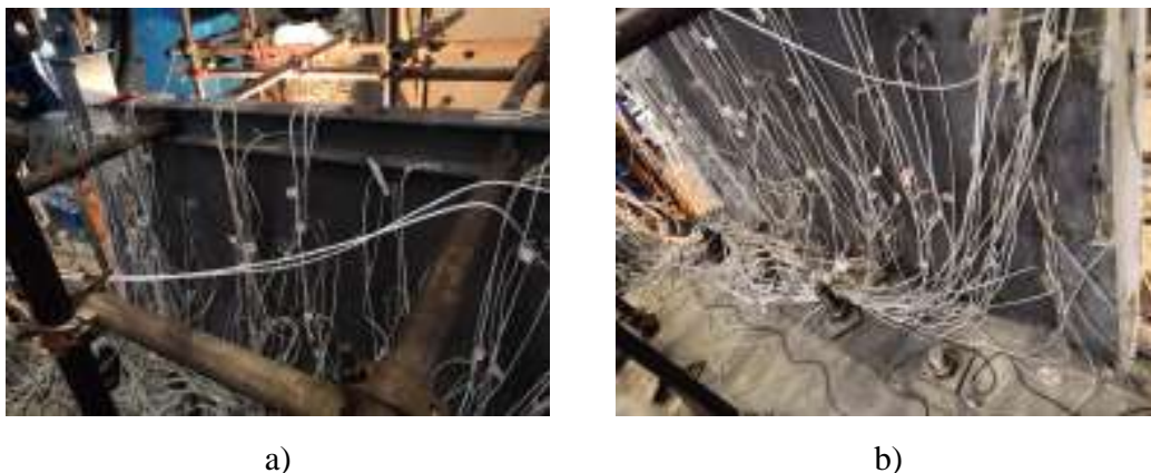
Fig. (8a,b). Arrangements of the strain gauges.
