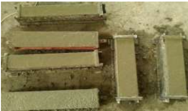
Fig. (7). Casting of flexural beam.
