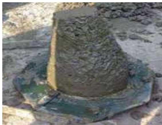
Fig. (4). Slump test.
