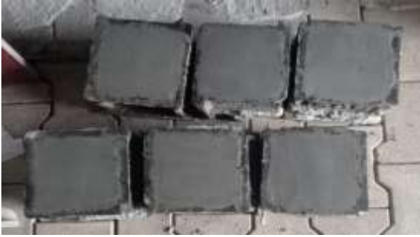
Fig. (6). Casting of concrete cubes.
