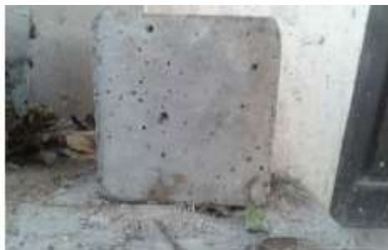
Fig. (10). Concrete cube after durability test.
