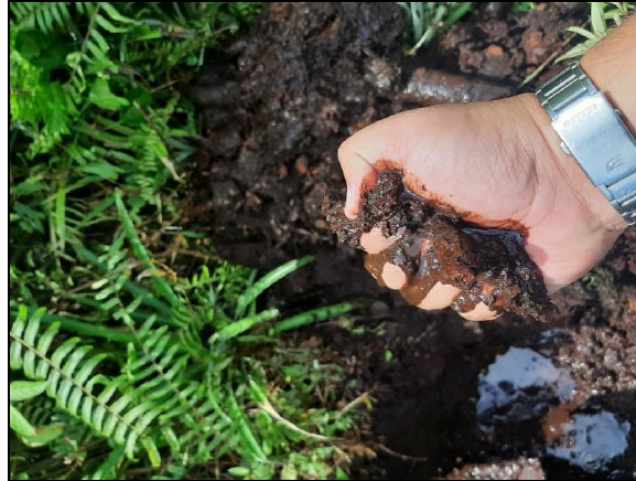
Fig. (3). Von-post test applying hand squeezing method.
