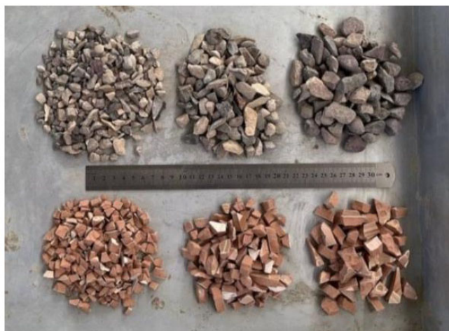
Fig. (2). Ceramic aggregate after crushing and grading (12.5 mm, 19 mm, 25 mm), Upper: Natural crushed stone, Lower: Coarse ceramic waste.
