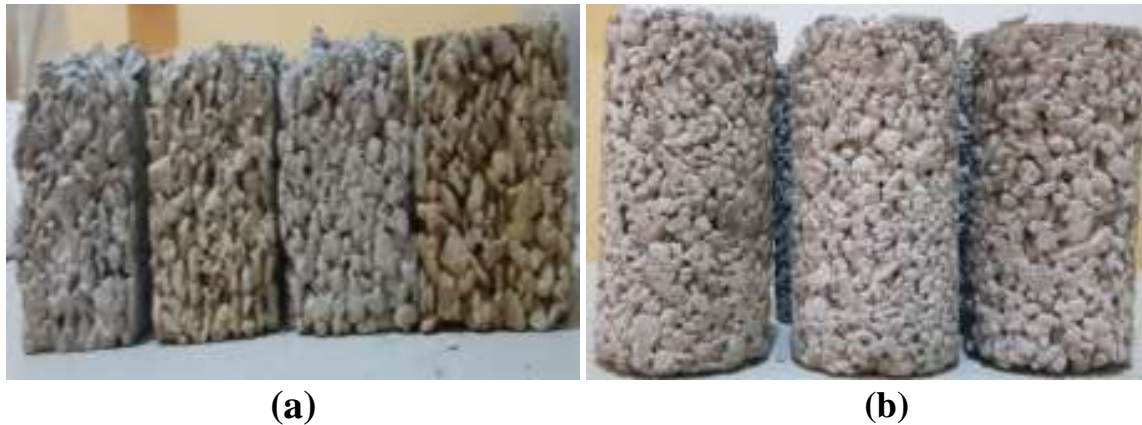
Fig. (3). Pervious concrete (a) Cubes for compressive strength test (b) Cylinders for split tensile strength test.
