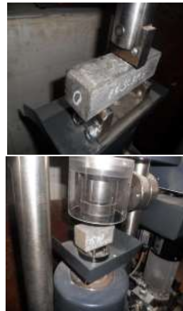
Fig. (3). Flexural and compressive strength test.
