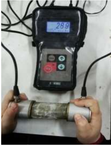
Fig. (4). The process of measuring the propagation velocity of ultrasonic waves through the specimen.
