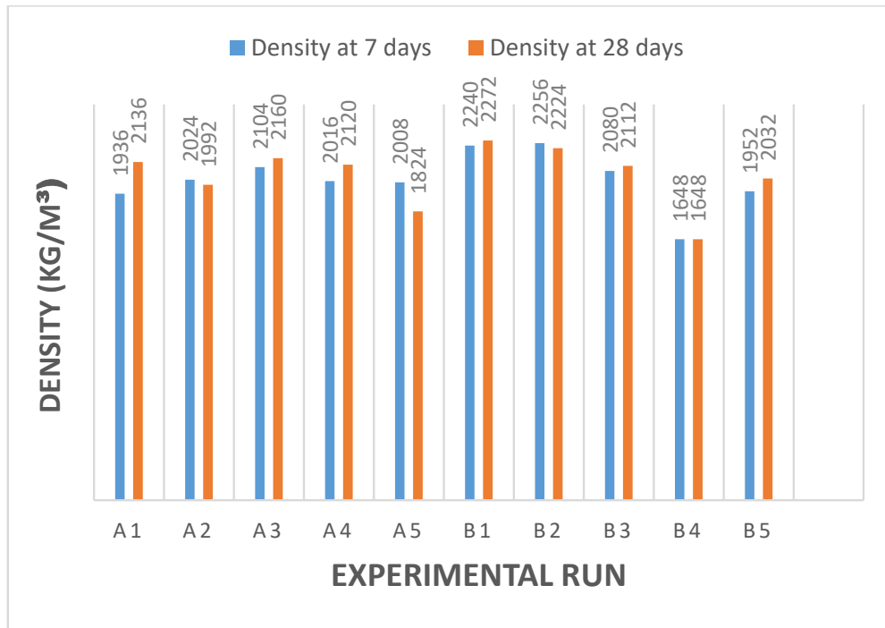
Fig. (9). Density of cement-wood ash mortar.
