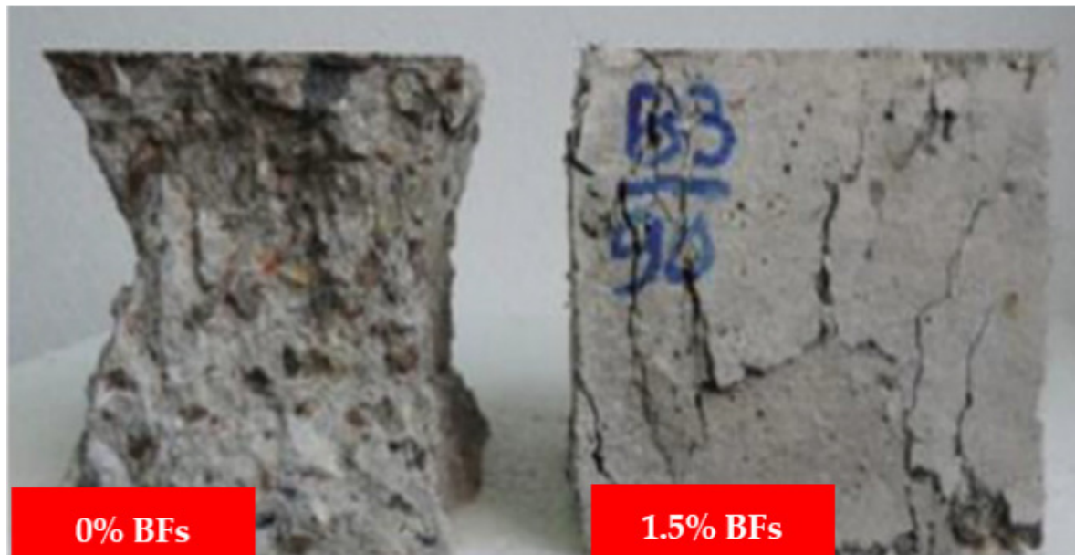
Fig. (2). Compressive failure modes.
