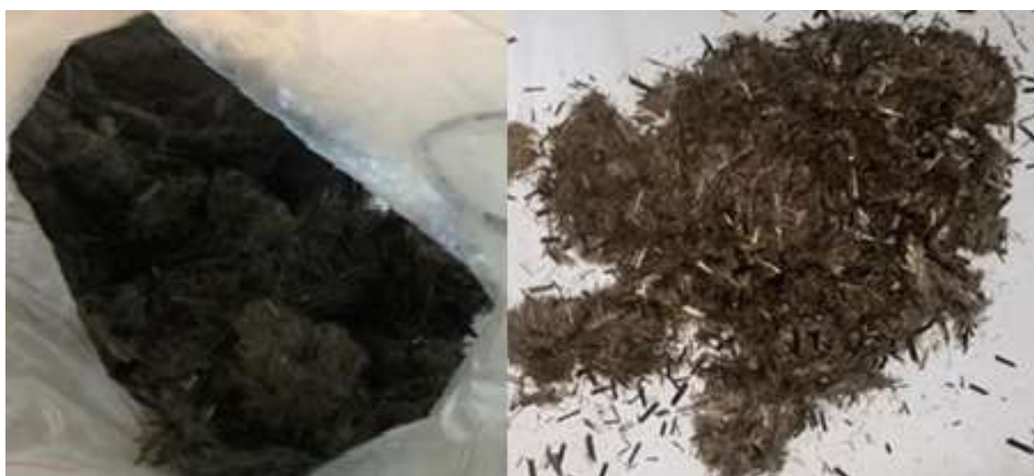
Fig. (3). Micro basalt fibers (soft chopped basalt fiber).
