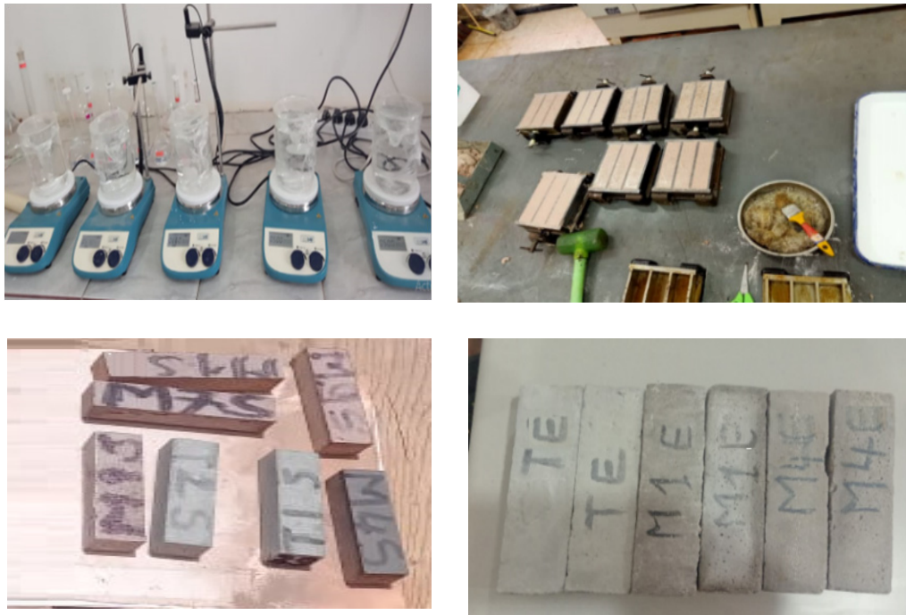
Fig. (2). The preparation of alkaline activators and metakaolin geopolymer mortars and curing regime.
