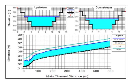
$\textbf{Fig. (8).} \ \ \text{Water level at the design cross-section, cross-section, and long section.}$
