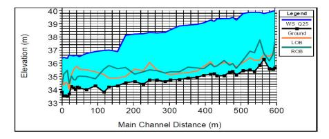
Fig. (6). Water level with plan flood at the existing cross-section.
