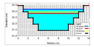
$\textbf{Fig. (10).} \ \ \text{Water level of cross-section plan with vetiver grass, shrub grass, and bamboo plants at the upstream.}$
