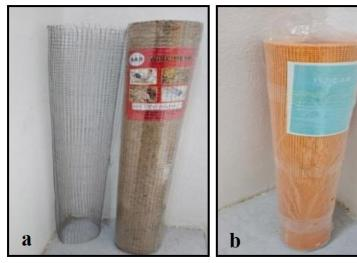
a. Welded Wire Mesh and b. Glass Fiber Mesh.
