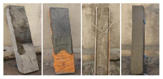
a) Filling Voids of Mesh b) Fixing Wood Rule c) Final Appearance
