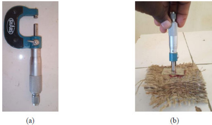
Fig. (4). Micrometer (a), measuring the thickness of a geotextile test sample (b).
