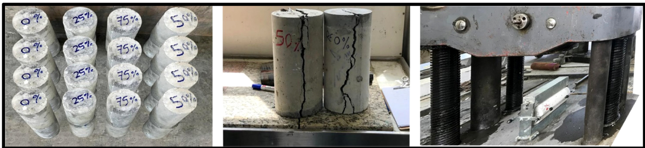
Fig. (4). Splitting tensile strength test of mixes (ASTM C496) [18].
