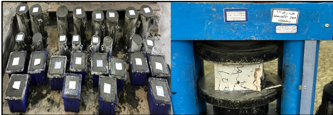
Fig. (2). Compressive strength test of RCA-HSF concrete at 28 days (tested per BS EN 12390-3:2019) [16].
