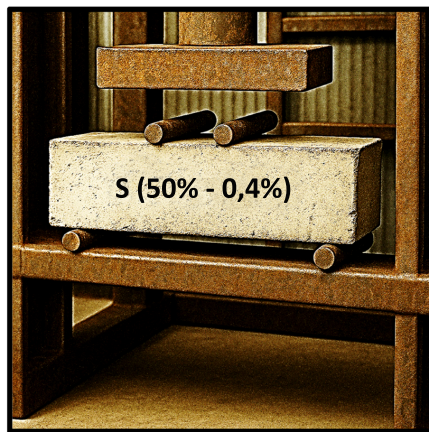
Fig. (3). Flexural strength test under third-point loading (ASTM C78) [17].
