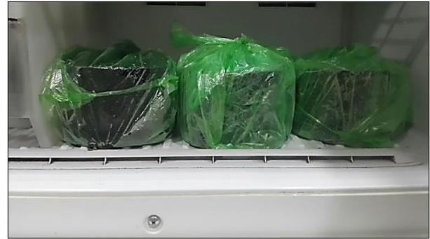
Fig. (18). Specimens freezing at -18^\circ\text{C} for 16 hours.
