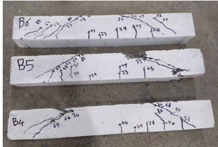
Fig. (5). Pattern of failure cracks of the beam specimens.
