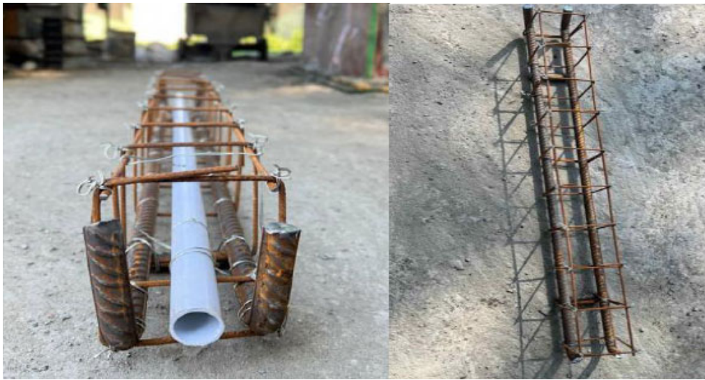
Fig. (2). Reinforced cage of beam specimens.
