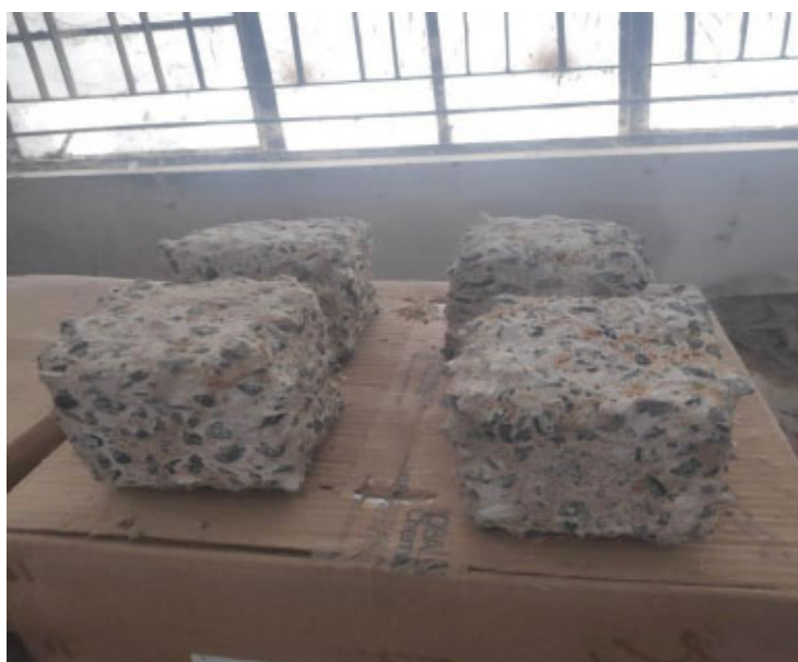
Fig. (12). Visual observation of concrete exposed to acid attack.
