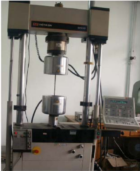
Fig. (4). Fatigue test setup.
