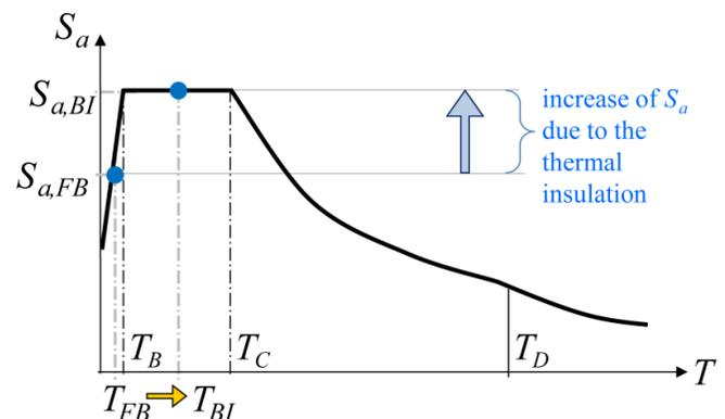
Fig. (2). Roof accelerations of the stiff superstructure in relation to its fundamental period – comparison of the fixed base (FB) and base isolated (BI) building.
