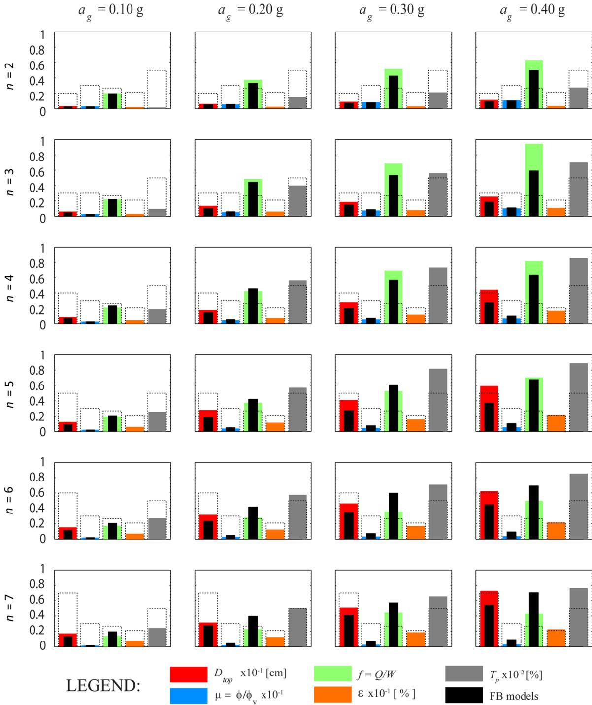
Fig. (6). The comparison of the fixed base (FB) and base isolated (BI) elastic ( $\alpha = 1.0$ ) building model response.
