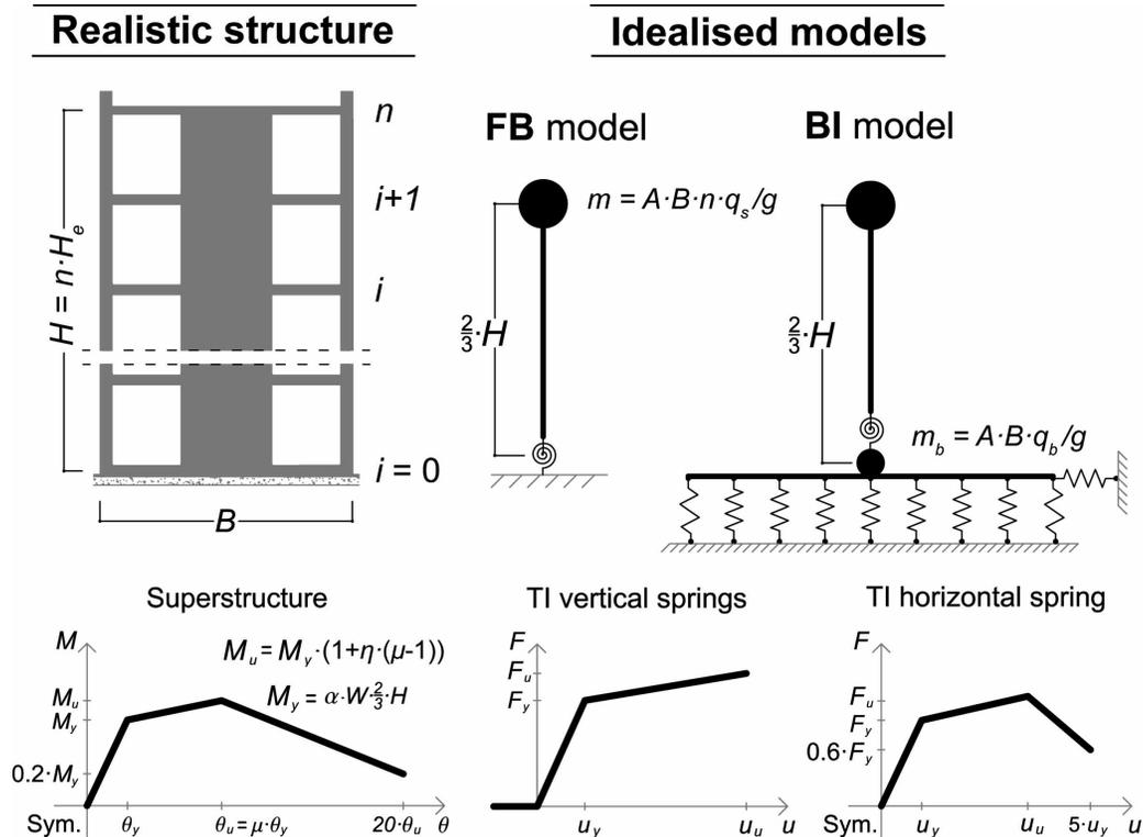
Fig. (3). Comparison of the fixed base (FB) and base isolated (BI) building model with nonlinear backbone curves.
