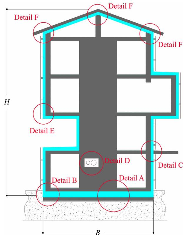
Fig. (1). Schematic representation of low-energy buildings' details critical from the point of view of earthquake resistance.
