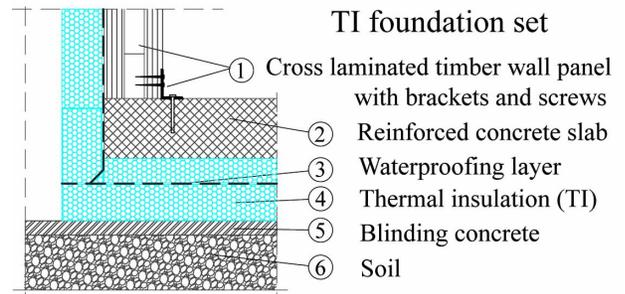
Fig. (4). The detail of a TI layer with XPS boards and inserted waterproofing (HI) foil.
