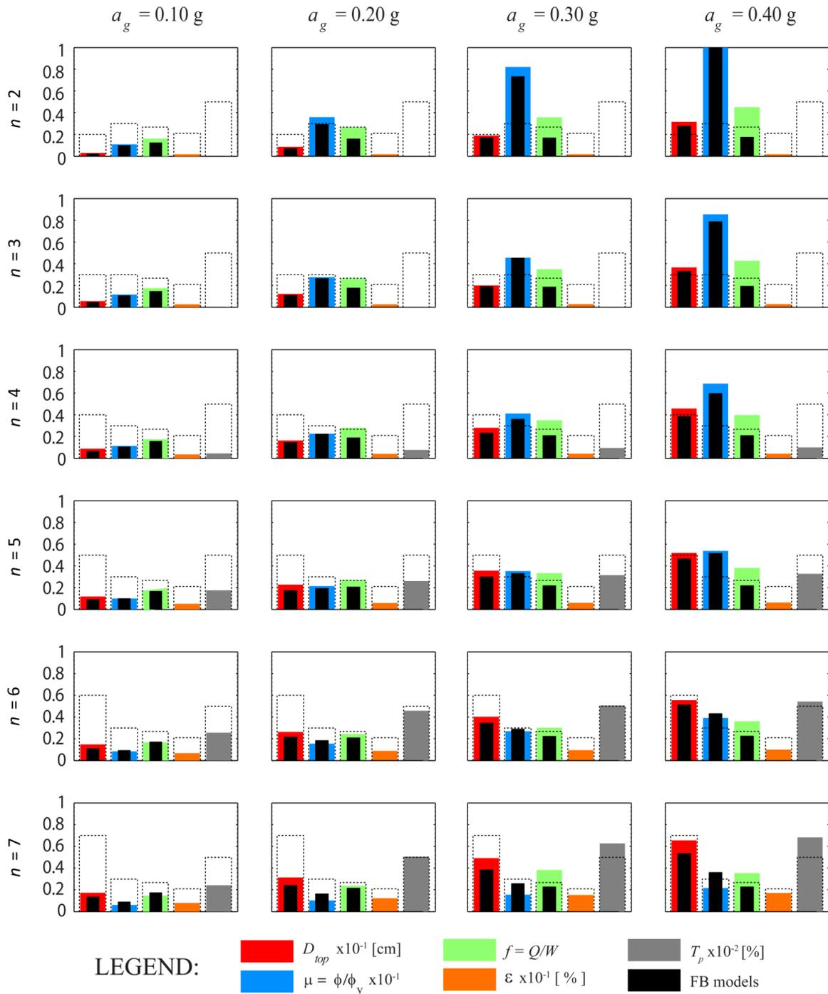
**Fig. (5).** The comparison of the fixed base (FB) and base isolated (BI) inelastic ( $\alpha = 0.25$ ) building model response.
