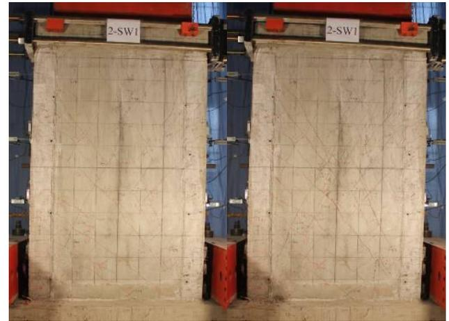
a. Crack pattern at peak load b. The drift ratio 1/70
