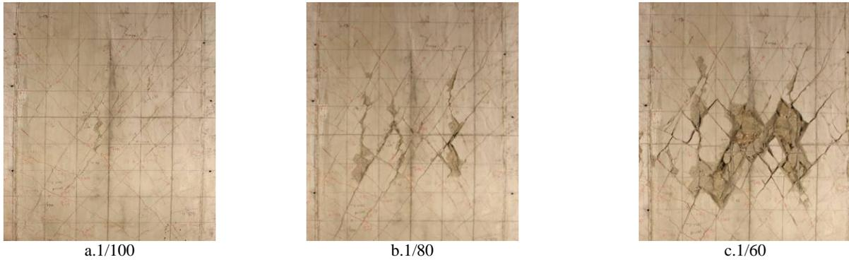
Fig. (10). Failure behaviors of 2-SW1 at three drift ratios.
