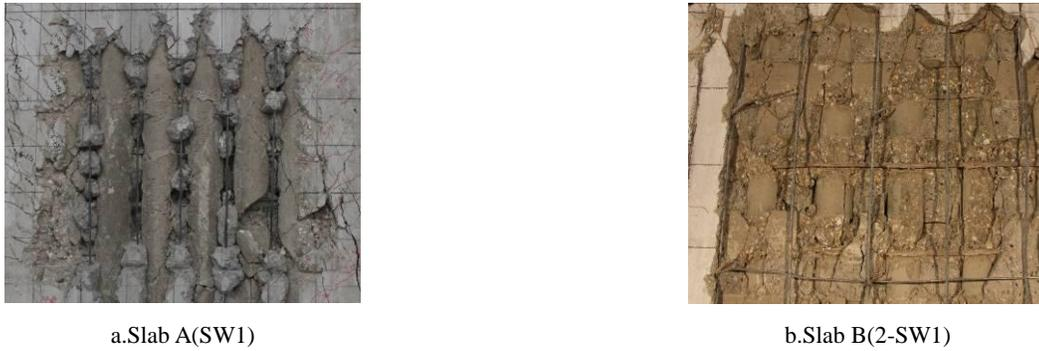
Fig. (11). Inner failure pattern of specimens.
