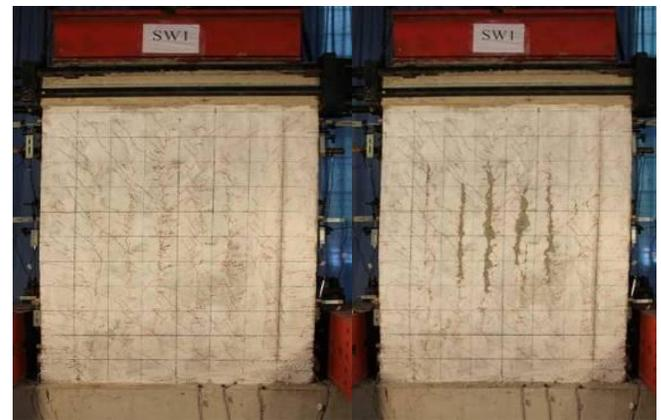
a. Crack pattern at peak load b. The drift ratio 1/100
