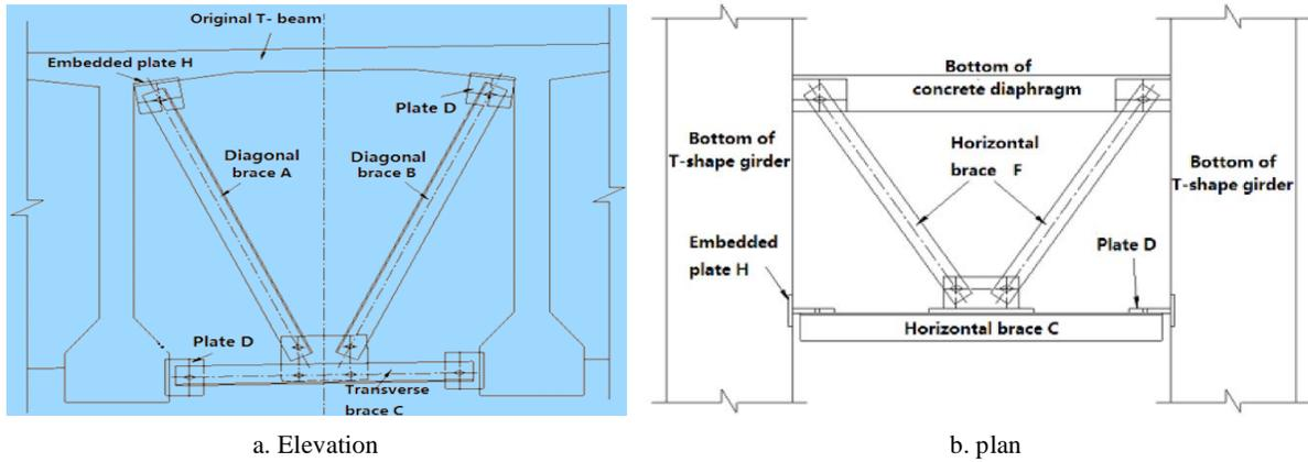
Fig. (4). Design of spacial Double-K shape brace.
