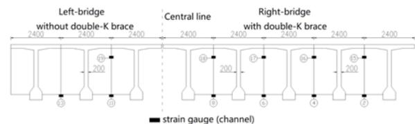
Fig. (10). Strain gauge displacement in the 1/3L diaphragms.
