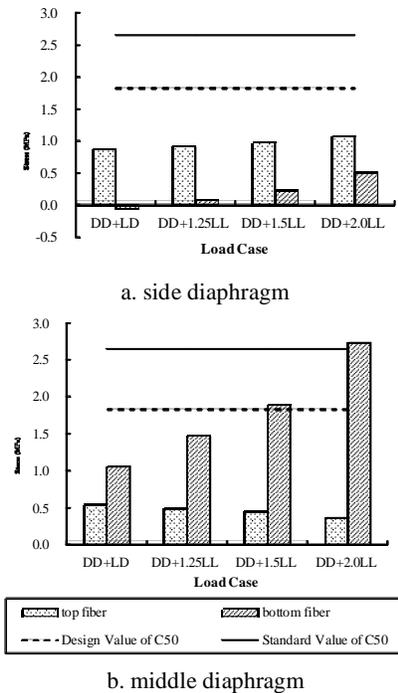
Fig. (3). Concrete stress of mid-span diaphragm under different live load
