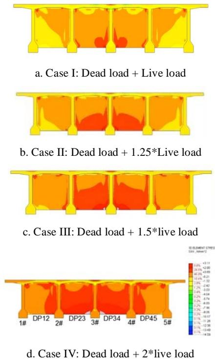
Fig. (2). Stress of concrete under different live load intensity.
