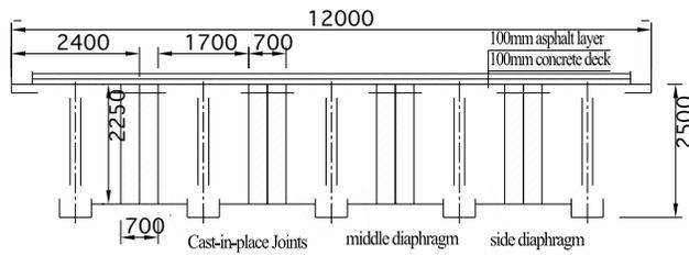
Fig. (1). Cross-section of background bridge.
