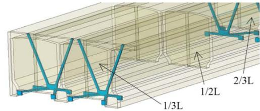
Fig. (6). FE model of bridge with double-K brace (partial view).
