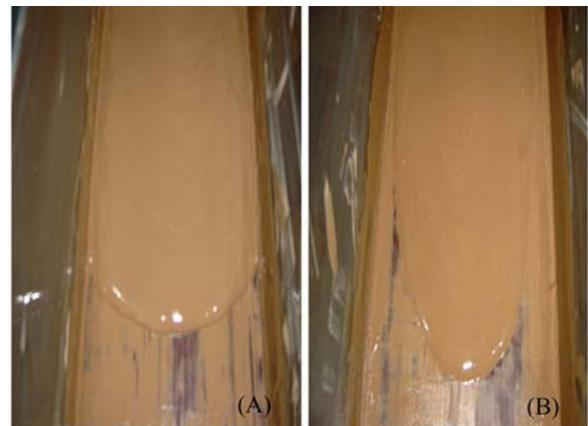
Notes: (A) Fixed bed and gentle slope (*i* = 5.5%,  $\gamma$  = 16.8 KN/m<sup>3</sup>); (B) Fixed bed and steep slope (*i* = 5.5%,  $\gamma$  = 16.8 KN/m<sup>3</sup>).
