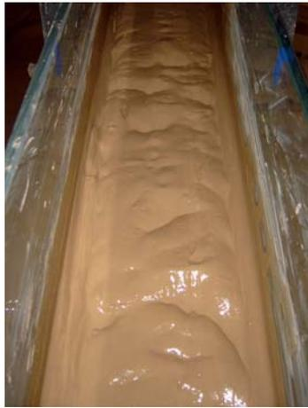
Notes: Fracture state of mud surface ( $\gamma = 17.5 \text{ KN/m}^3$ ,  $i = 14.0\%$ ,  $Q=1.50\text{l/s}$ ).
