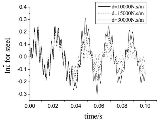
Fig. (7). Variations of strain rate for steel versus time.
