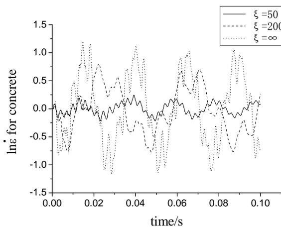
Fig. (4). Variations of strain rate for concrete versus time.
