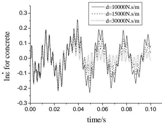
Fig. (6). Variations of strain rate for concrete versus time.
