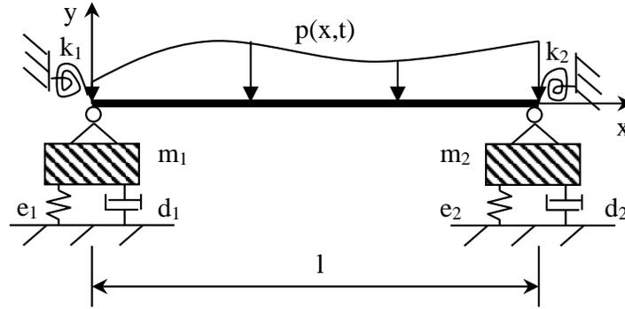
Fig. (1). Analytical model for beam with flexible supports.
