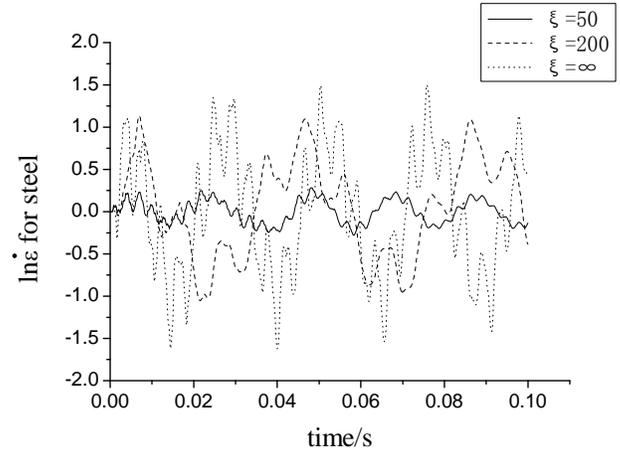
Fig. (5). Variations of strain rate for steel versus time.
