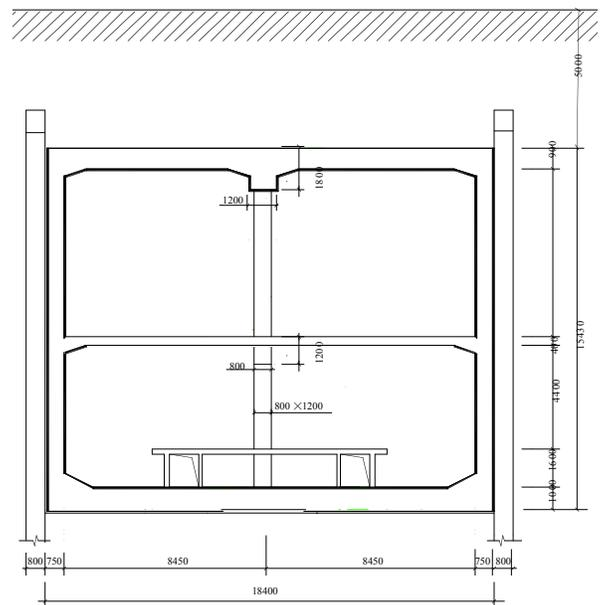
Fig. (1). The section plane of subway station.
