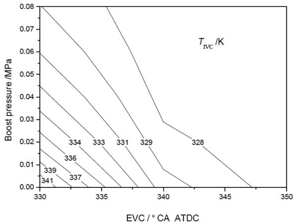
Fig. (4). Effects of EVC and boost pressure (gauge) on  $T_{IVC}$ .
