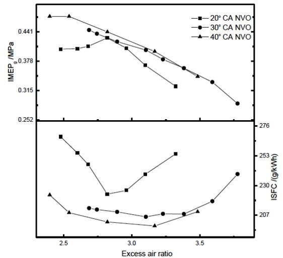
Fig. (9). (a) Effect of  $\alpha$  on IMEP<sub>g</sub> and ISFC of HCCI Combustion at Various NVOs.
