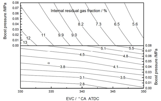
Fig. (3). Effects of EVC and boost pressure (gauge) on IEGR.
