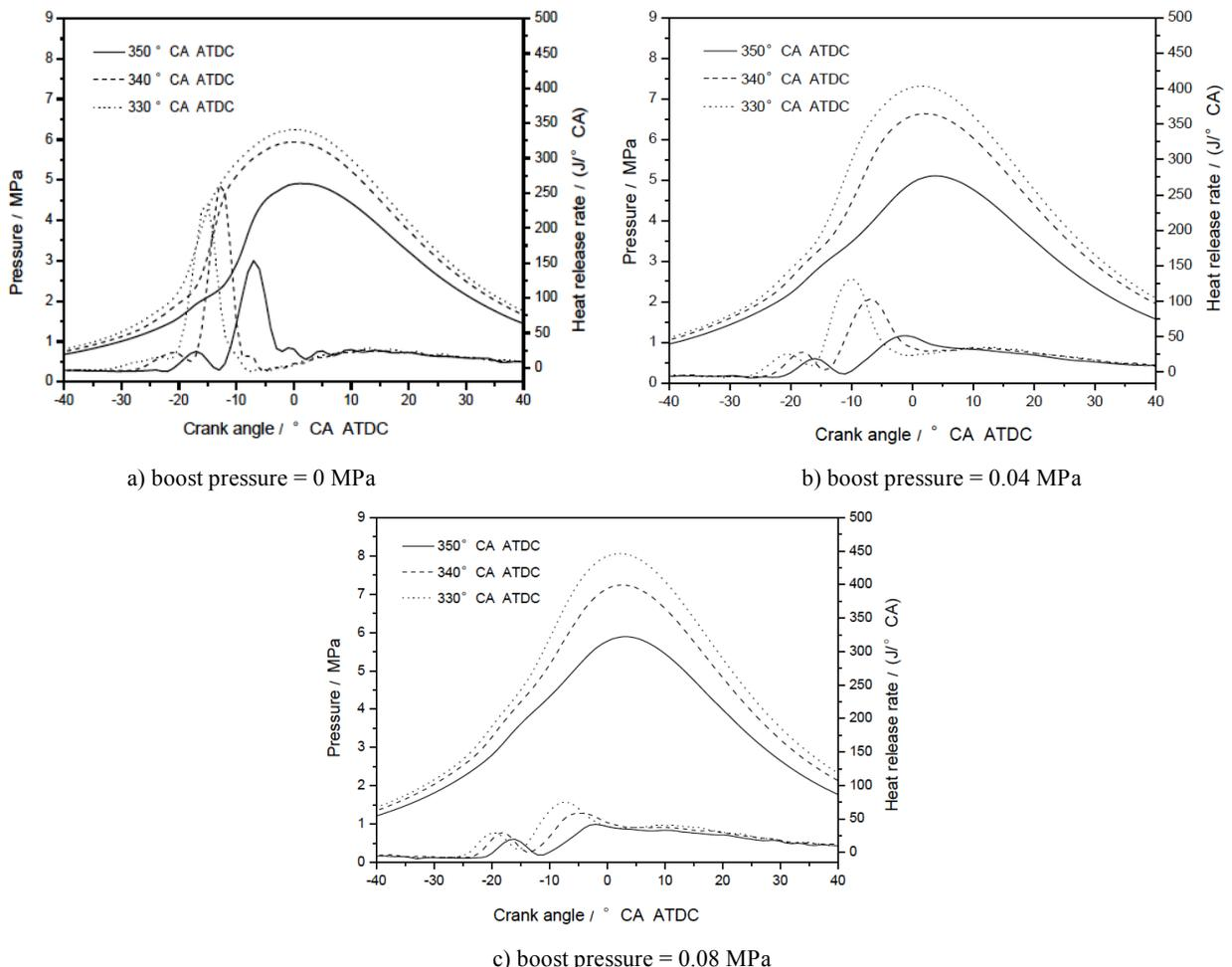
Fig. (5). Effects of EVC on cylinder pressure and heat release rate at various boost pressures (gauge).
