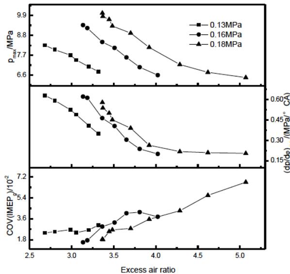
Fig. (12). Effect of excess air ratio on HCCI limit at various boost pressures.
