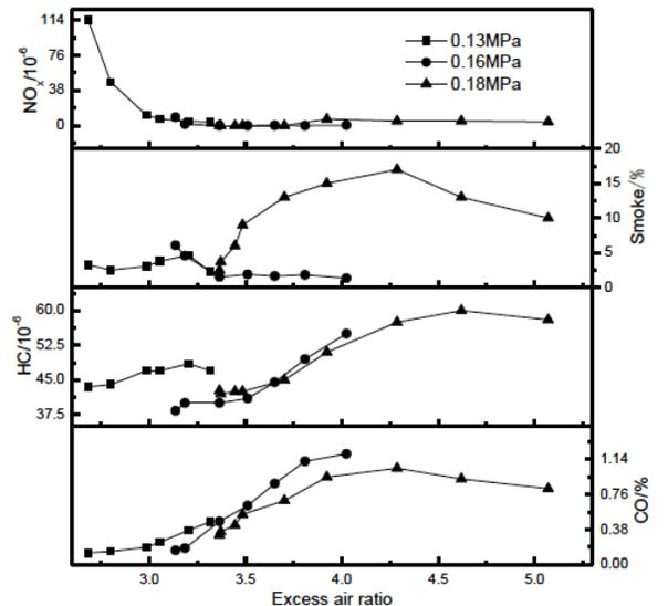
Fig. (10). (b) Effect of  $\alpha$  on HCCI emission at various boost pressures.
