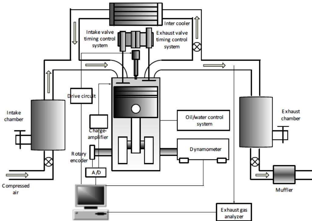
Fig. (1). Schematic diagram of the test system.
