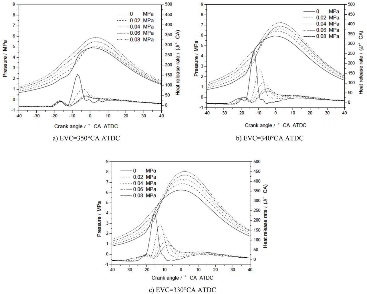
Fig. (6). Effects of boost pressure (gauge) on cylinder pressure and heat release rate at various EVCs.
