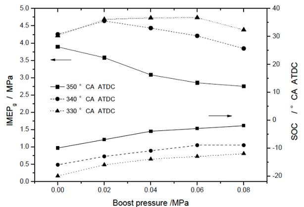
Fig. (7). Effects of EVC and boost pressure (gauge) on IMEP<sub>g</sub> and SOC.
