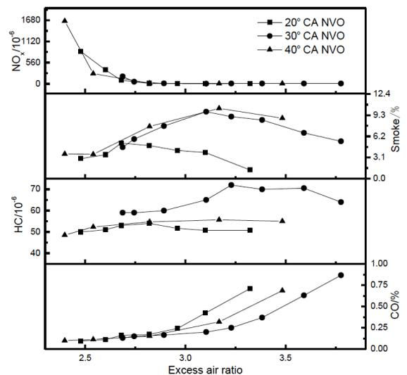
Fig. (9). (b) Effect of  $\alpha$  on emissions of HCCI combustion for various NVOs.
