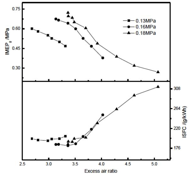
Fig. (10). (a) Effect of  $\alpha$  on IMEP<sub>g</sub> and ISFC of HCCI combustion at various boost pressures.
