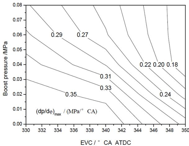
Fig. (8). Effects of EVC and boost pressure (gauge) on  $dp/d\phi_{max}$
