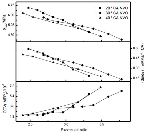
Fig. (11). Effect of excess air ratio on HCCI limit at various NVOs.
