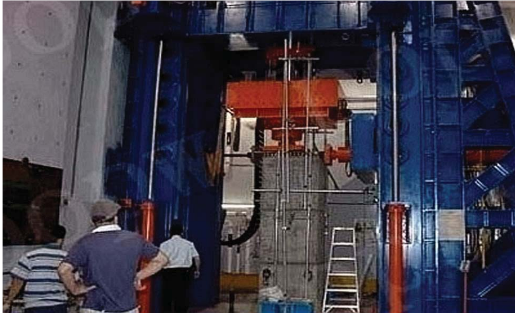
Fig. (3). Large multifunctional structural testing system.
