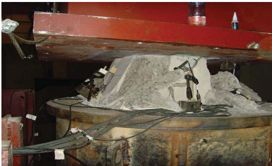
Fig. (6). The axial compression performance test of brittleness specimen.
