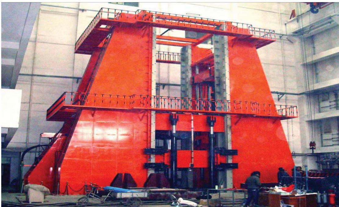
Fig. (5). Multifunctional structure loading system (40000kN).
