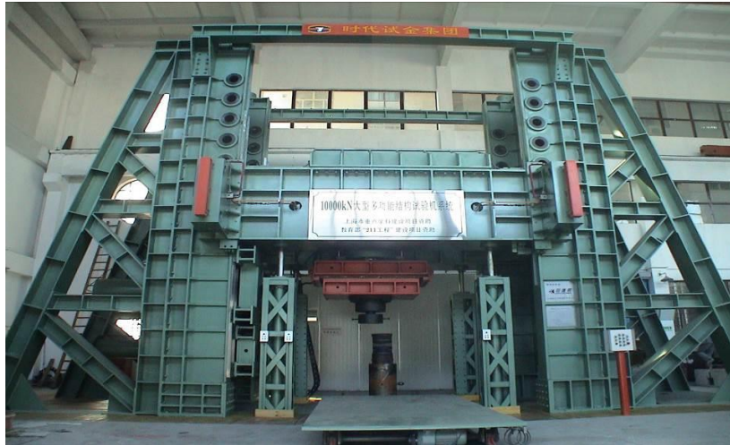
Fig. (1). Large multifunctional structural experiment system.
