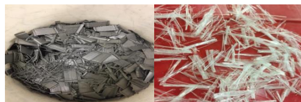
Fig. (2). Steel fibres (left) and PP fibres (right).
