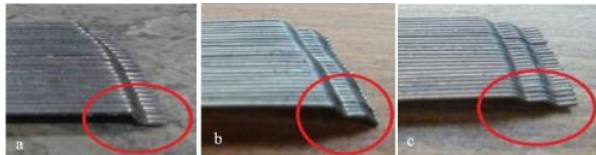
Fig. (1). Hooked-end steel fibres (Reprinted from (Okeh, Begg et al. )
