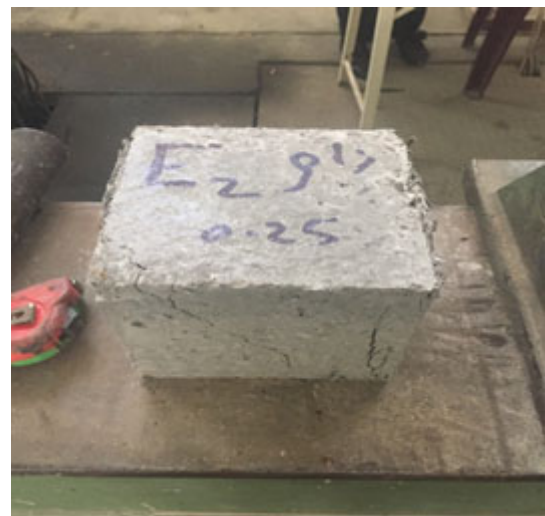
Fig. (12). Failing pattern of PFRC under compression test.
