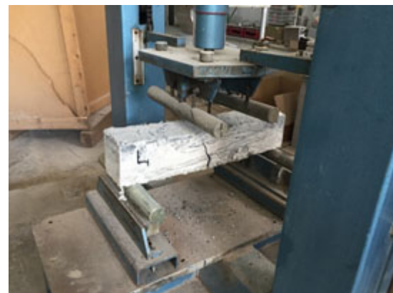
Fig. (17). Failing pattern of Hybrid fibers reinforced concrete under flexural strength test.
