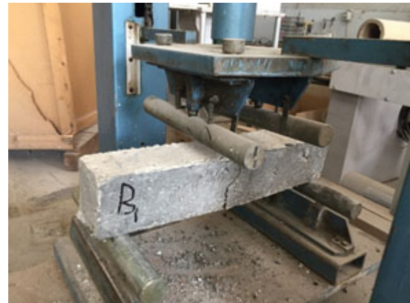
Fig. (16). Failing pattern of polypropylene fibers reinforced concrete under flexural strength test.
