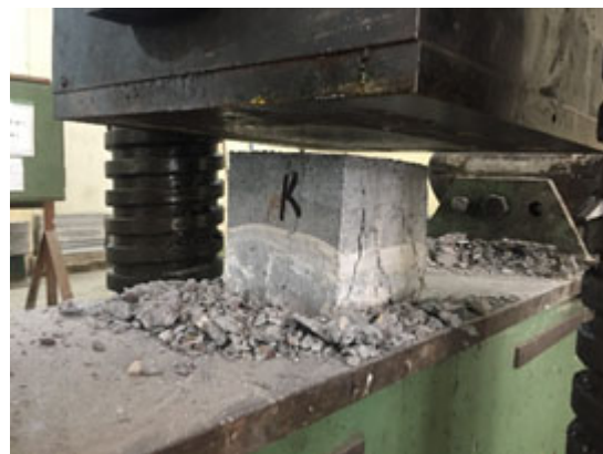
Fig. (13). Failing pattern of HFRC under compression test.
