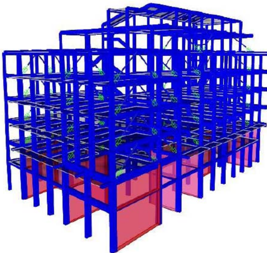
Fig. (19). 3D model of the building retrofitted using RC walls and damped braces.
