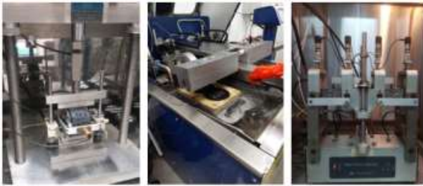
Fig. (2). Tests of Asphalt Mixture with UMATTA, HWTD, and BFA.
