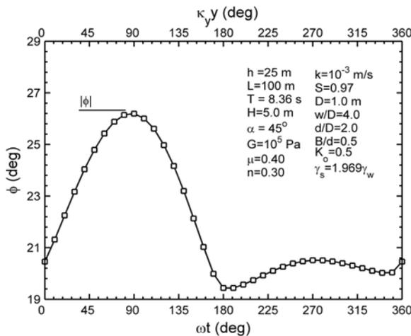
**Fig. (12).** The distribution of stress angle for a point located on the pipe perimeter at  $\theta=135^\circ$  (a) over a pipeline span axis, when  $t=T$  (see the upper horizontal axis:  $\kappa_y$ ), (b) over a wave period, when  $y=0$  (see the lower horizontal axis:  $\omega t$ ).
