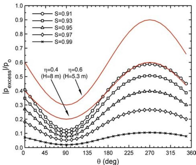
Fig. (19). Variations of  $|p_{excess}|/p_o$  with soil saturation.
