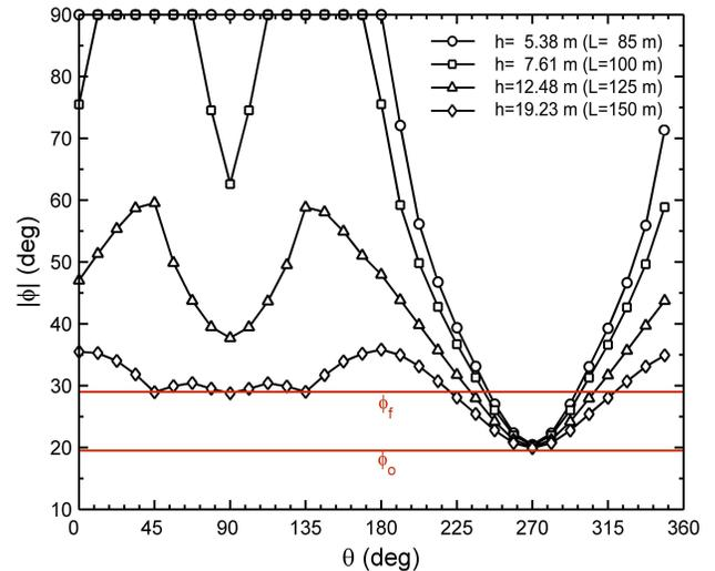
Fig. (33). The distribution of  $|\phi|$  around pipeline for various water depths.
