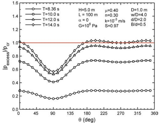
Fig. (29). The potential of soil liquefaction around pipe perimeter for various  $T$ . ( $K_o = 0.5$  and  $\gamma_s = 1.969\gamma_w$ ).
