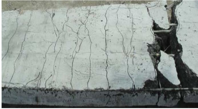
Fig. (13). Crack pattern of GFRP 2 reinforced slab.
