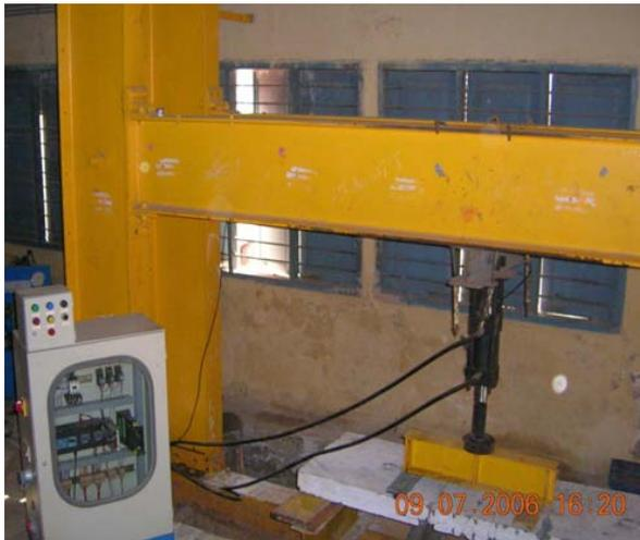
Fig. ( 3). Experimental setup for fatigue loading.
