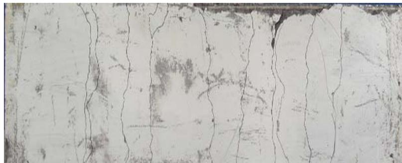
**Fig. (12).** Crack pattern of GFRP 1 reinforced slab.
