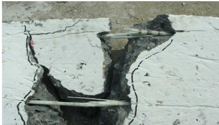
Fig. (14). Failure of GFRP slabs: Concrete crushing followed by the rupture of GFRP reinforcements.
