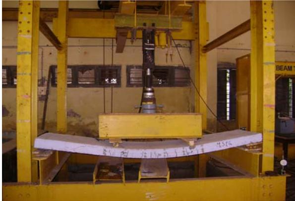
Fig. (1). Experimental setup for testing the slabs.
