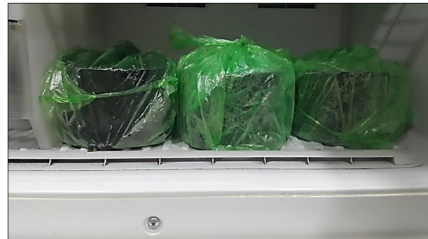
Fig. (18). Specimens freezing at -18^\circ\text{C} for 16 hours.
