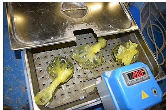
Fig. (19). Specimens in a 60^\circ\text{C} water bath for 24 hours.
