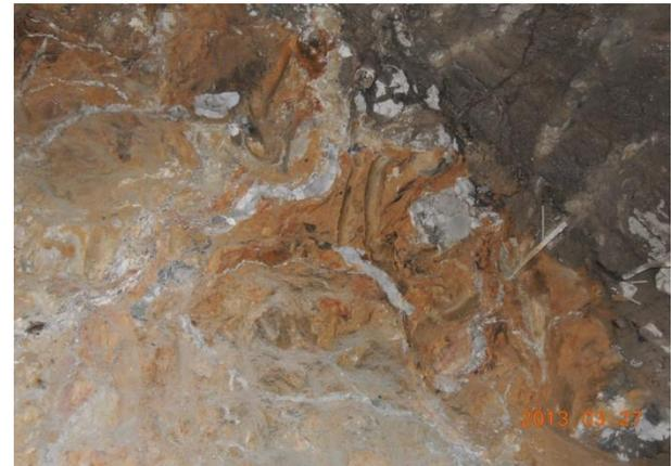
Fig. (19). Slurry veins exposed by excavation.
