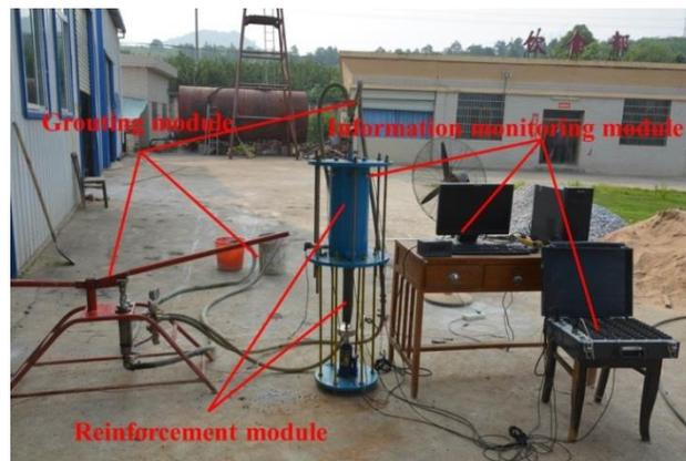
Fig. (9). Structure of model experiment device
