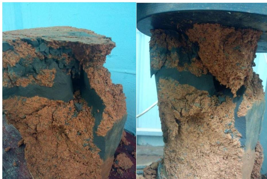
Fig. (11). Slurry veins inside the medium.
