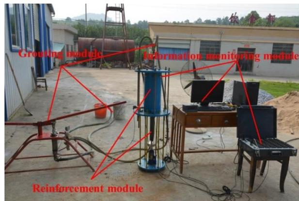
Fig. (9). Structure of model experiment device
