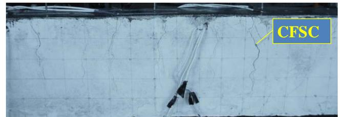
(a) Critical flexure-shear crack (CFSC).
