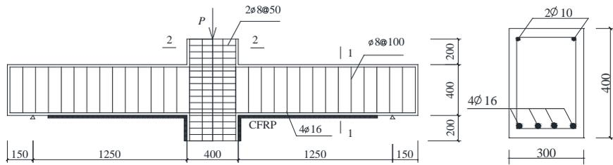
Fig. (3). Dimensions and reinforcement arrangement of B1e, B2e, and B2i.
