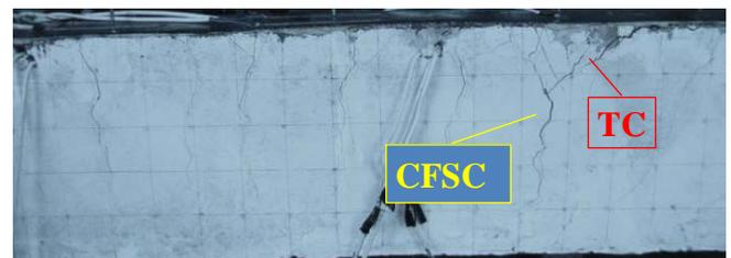
(b) Tributary crack (TC) initiated near the tip of CFSC.
