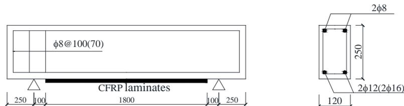
**Fig. (1). Dimensions and reinforcement arrangement of specimen.**
