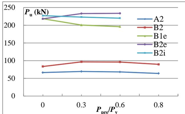
Fig. (7). Effect of preload level on ultimate load-carrying capacity.
