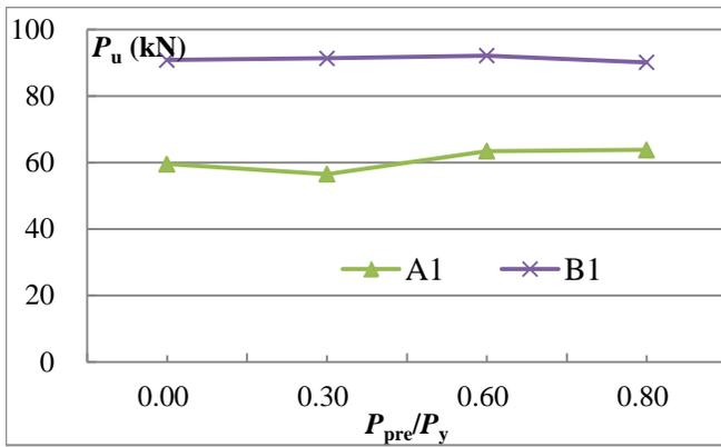
Fig. (6). Effect of preload level on ultimate load-carrying capacity.
