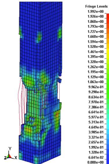
Fig. (5). Damage of column in 10kg TNT case.
