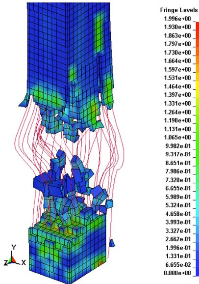
Fig. (6). Damage of column in 30kg TNT case.
