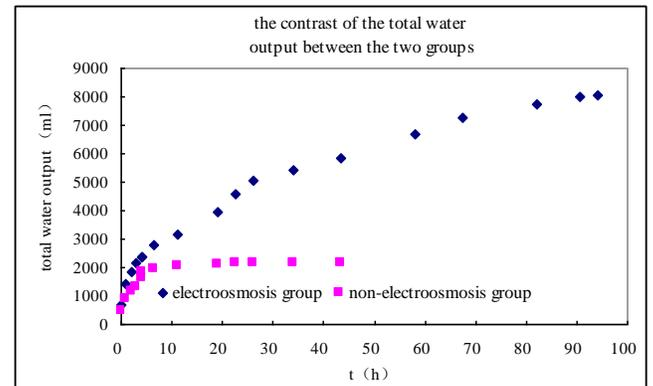
Fig. (12). The contrast of the total water output between the two groups.
