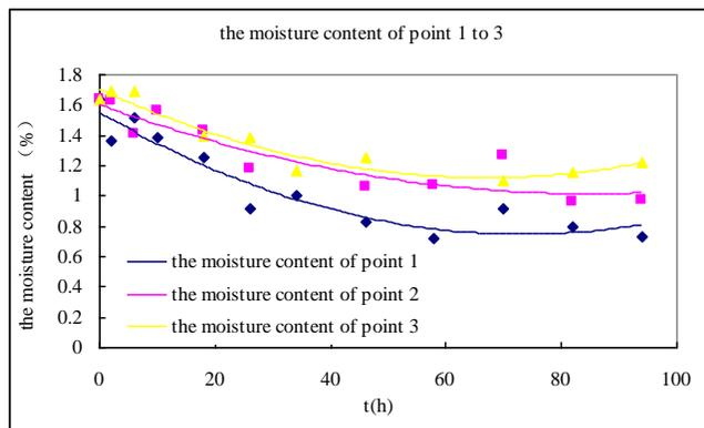
Fig. (7). The changes of moisture content with time at the surface of sludge.
