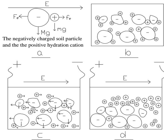
Fig. (9). The process of electro-osmosis dewatering.
