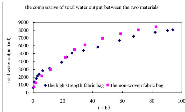
**Fig. (13).** The contrast of the total output water between the two materials.
