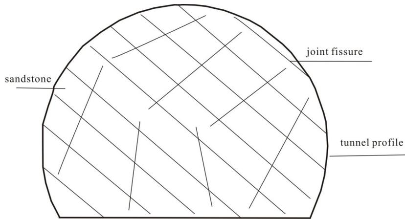
**Fig. (3).** Geological Sketch Of Tunnel Face On D2k31+821.
