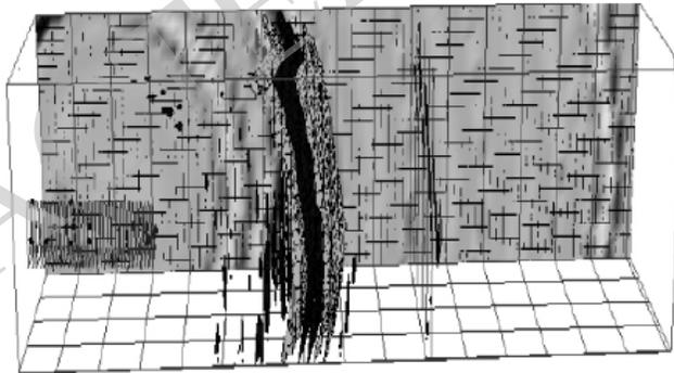
**Fig. (5).** Advanced Geological Prediction Of TRT6000 (Lateral).
