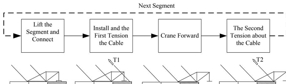
Fig. (2). Construction process of a standard girder.
