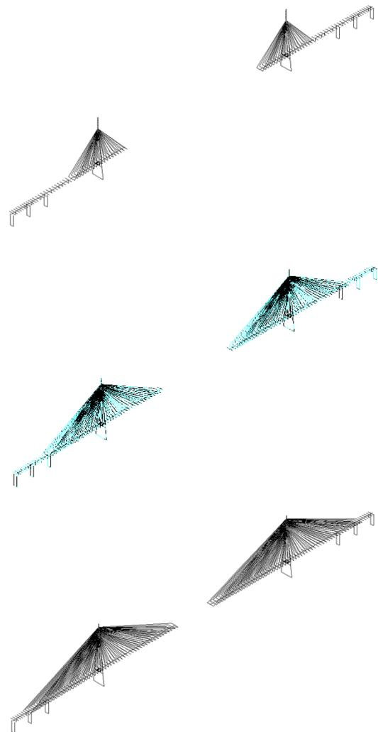
**Fig. (6).** FEA model of the construction stage.
