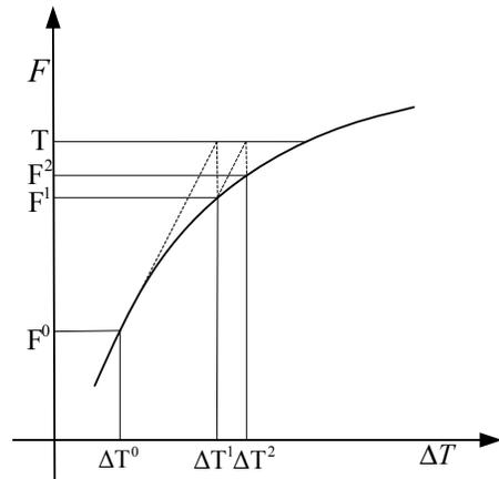
Fig. (1). Inclined cable tension iteration method.
