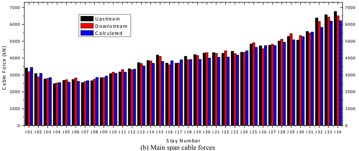
Fig. (9). Inclined cable force at the completed stage (kN).
