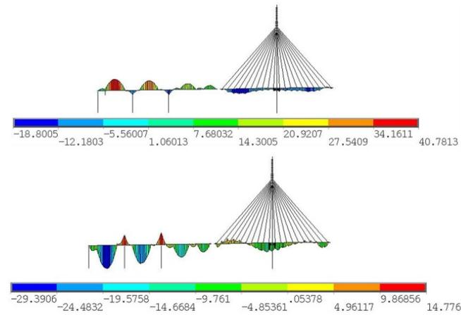
(a) Maximum double cantilever stage (no. 103 stage)
