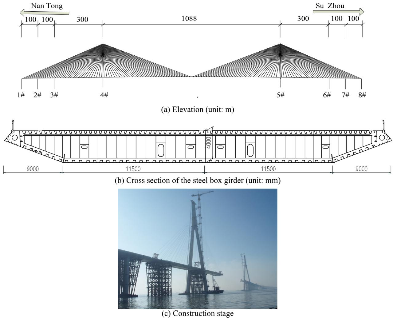
Fig. (4). Configuration of the Sutong Bridge.
