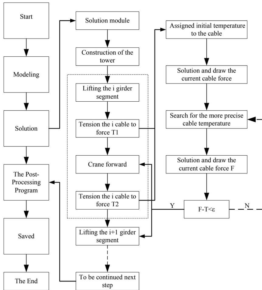
Fig. (3). Construction process simulation of a cable-stayed bridge.
