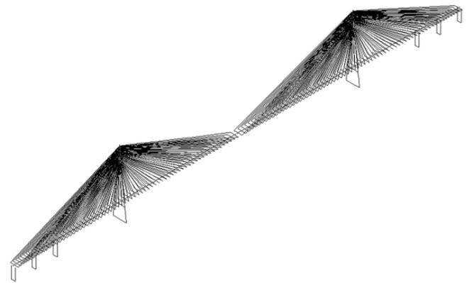
Fig. (5). Finite element model of the Sutong cable-stayed bridge.
