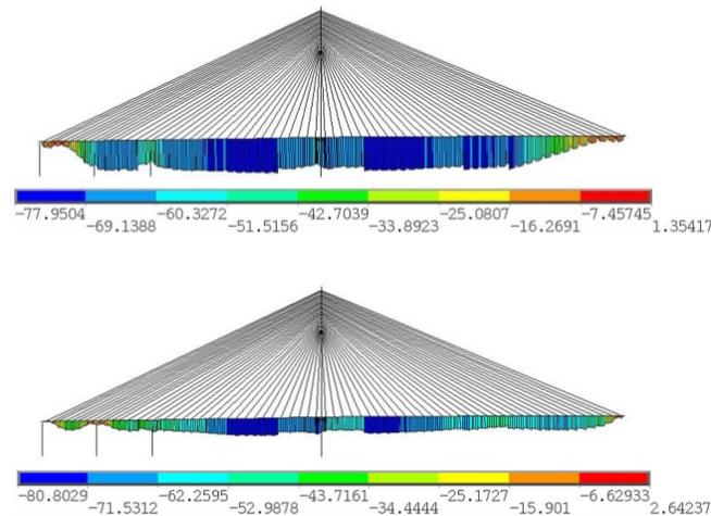
(b) Maximum single cantilever stage (no. 309 stage)
