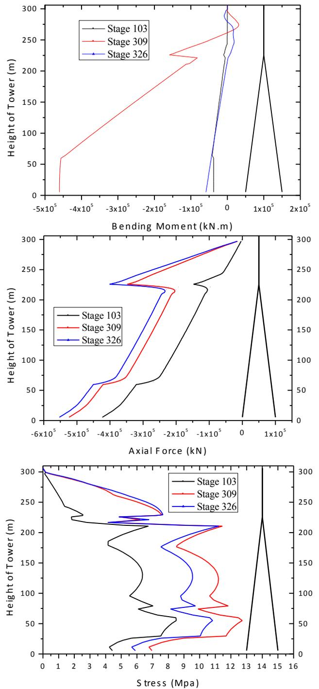
**Fig. (8).** Results of the tower at various stages of construction.
